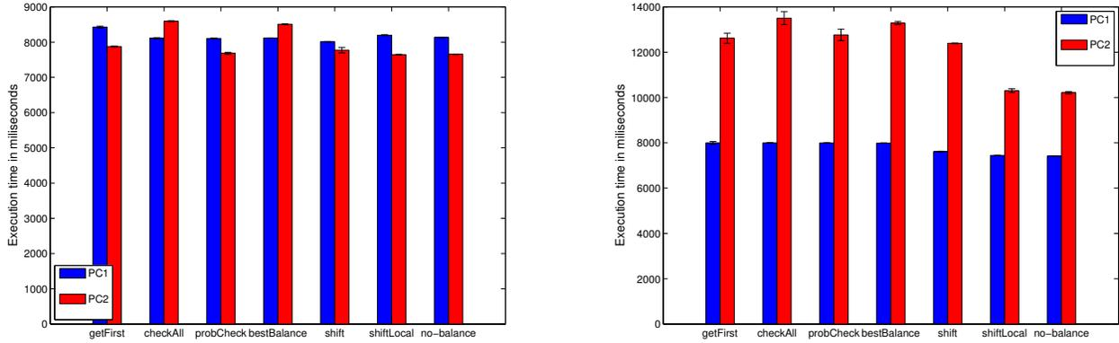
Figure 11: Comparison of execution time of load-balancing methods for DS3 (low imbalance) with grid size 4 (left) and 64 (right).
