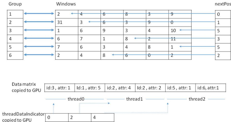
**Figure 2: Auxiliary data structures on the GPU.**
