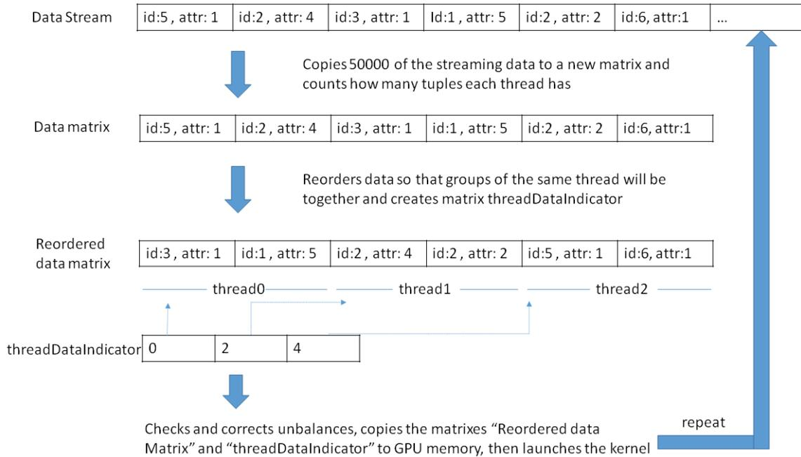
**Figure 1: High level data flow and CPU operations.**
